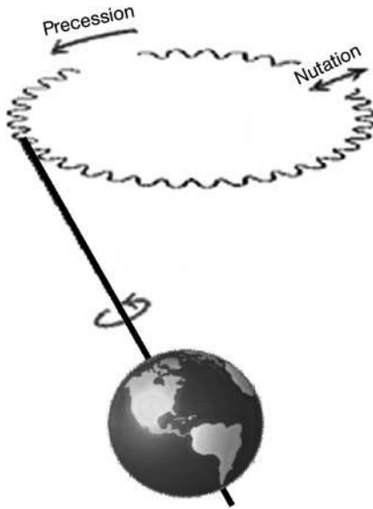
Figure 5.3 Schematic representation of precession and nutation.
