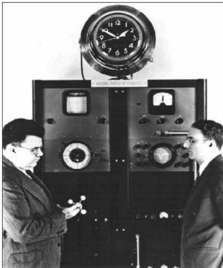
Figure 10.6 The first ammonia standard. The inventor, Harold Lyons, is on the right and the Director of the National Bureau of Standards, Edward Condon, is on the left (Lombardi, Heavner and Jefferts, 2007).
